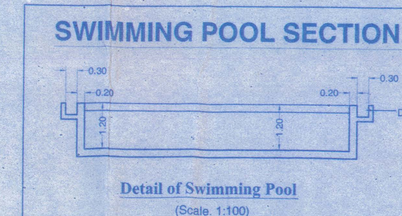
SWIMMING POOL SECTION (Scale: 1:100)
