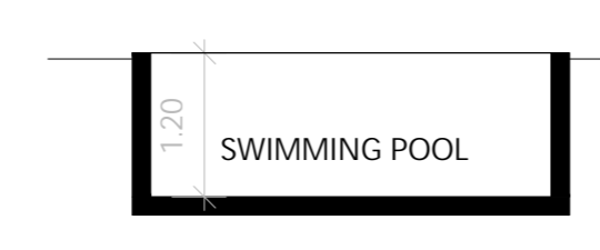
CROSS SECTION OF SWIMMING POOL (SCALE:- 1:100)
