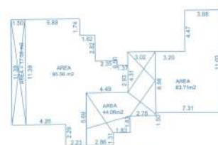
BLOCK-D1 AREA DIAGRAM OF UPPER GROUND FLOOR TOTAL BUILT UP AREA = 327.24m 2 deduction area of stair case = 44.00 m 2 deducted area of balcony = 23.91m 2 AREA FOR FAR- = 159.27m 2 Infrastructure Tax = 227.24m 2
