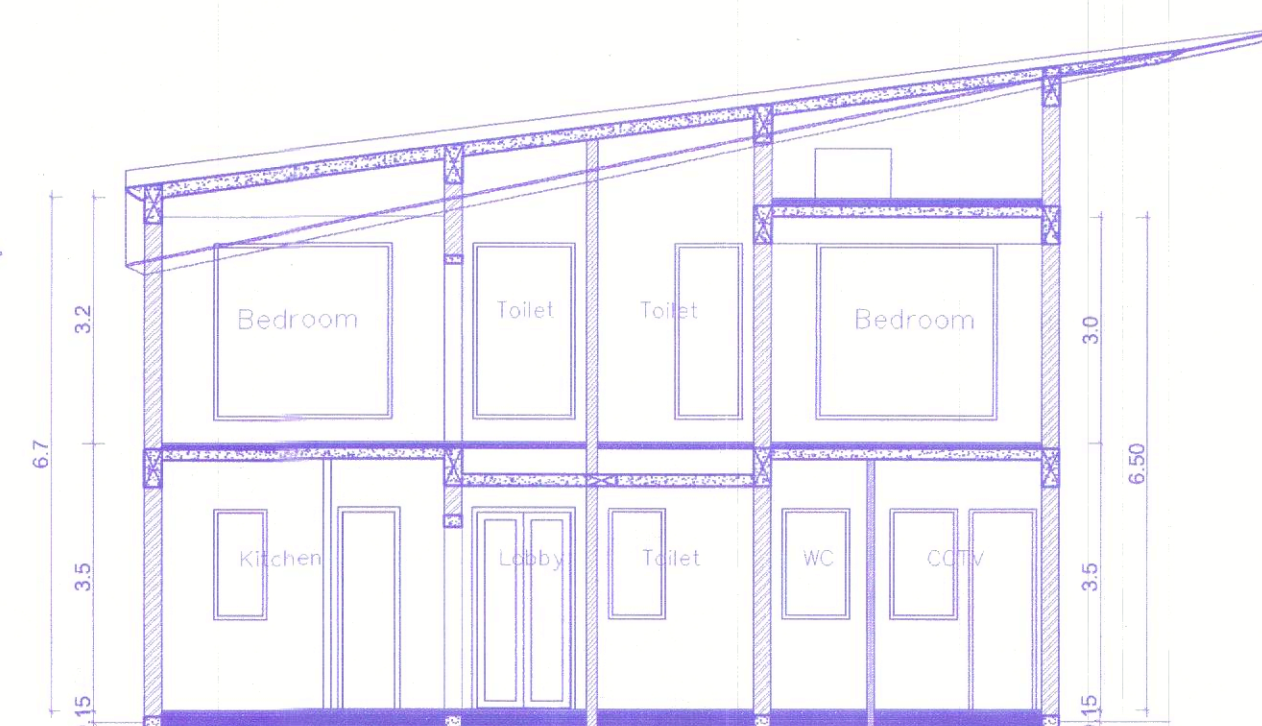
SECTION BB' Scale:- 1:100
